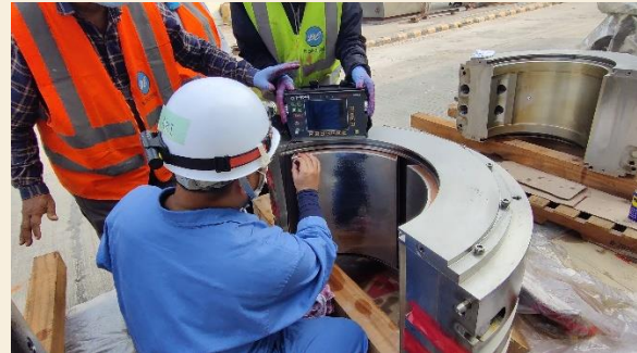
Figure: Ultrasonic Testing of GT Journal Bearing
